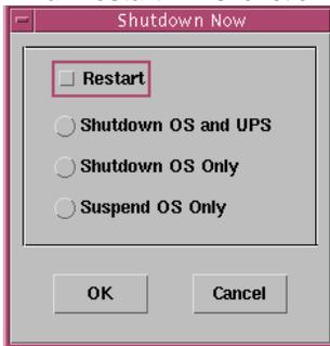
**b. Shutdown OS and UPS:** Use this function to shutdown both OS and UPS.
