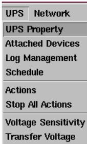
**UPS Property:** This dialog box allows you to configure the UPS COM port, battery replacement date,... etc. Load Warning and Load Severity are used to prevent UPS overload (see the UPS hardware user's manual). Load Warning will notify the user to reduce the load of the UPS. Load Severity will shutdown the computer to prevent overload.
