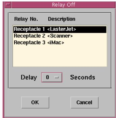
**Turn Receptacle Relay Off:** Turn the receptacle relay off. Each Receptacle Relay may control not only one outlet, please see the rear panel of your UPS or the UPS hardware user's manual.
