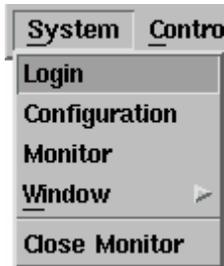
**Login:** Used for Remote Monitor. User must pass the password verification before he/she can control or configure the UPS.
